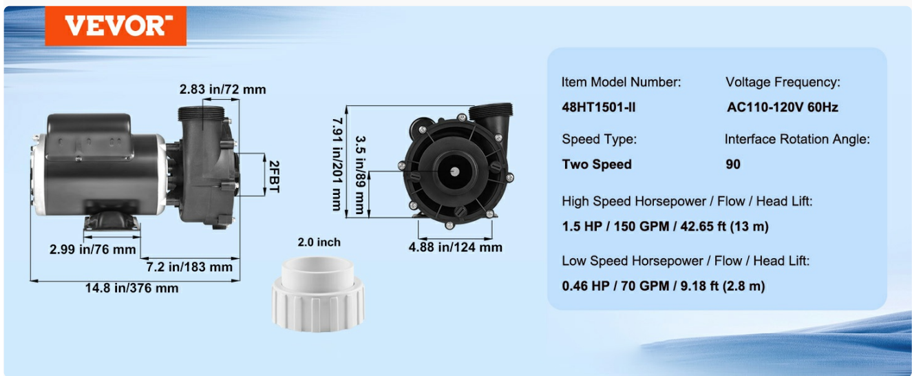
Image: Comprehensive diagram showing the dimensions and key specifications of the VEVOR 2 Speed SPA Pump.
