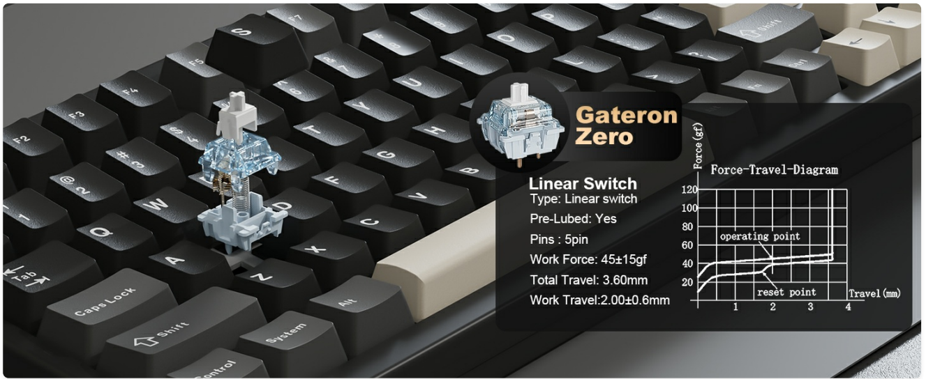
Image: Detailed specifications for the Gateron Zero Linear Switch, including type, pre-lubed status, pins, work force, total travel, and a force-travel diagram.
