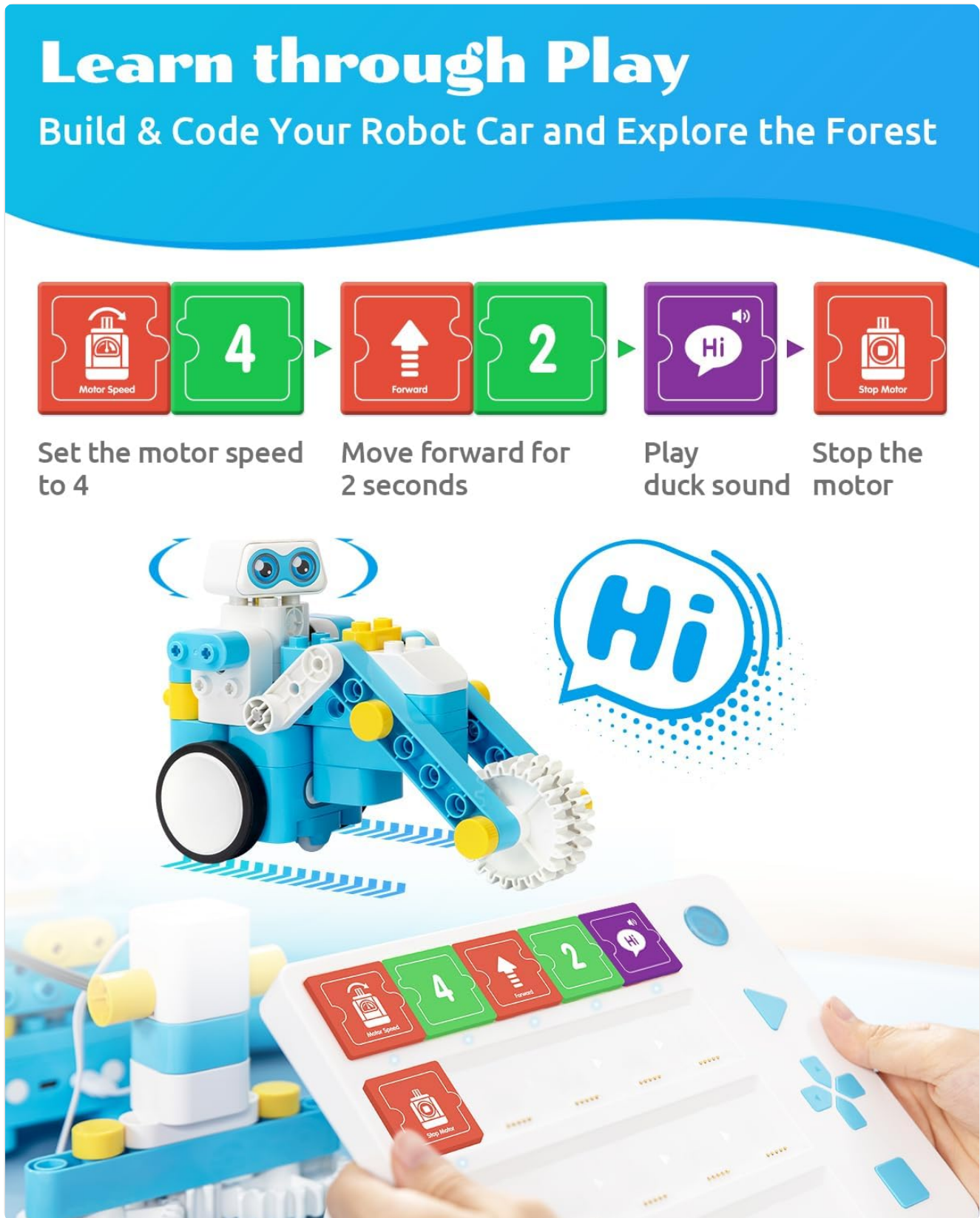
Figure 5: An example of a coding sequence using magnetic cards to set motor speed, move forward, play a sound, and stop the motor.
