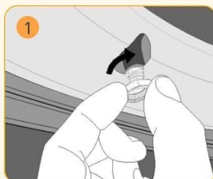
Installation of anti-theft nut
