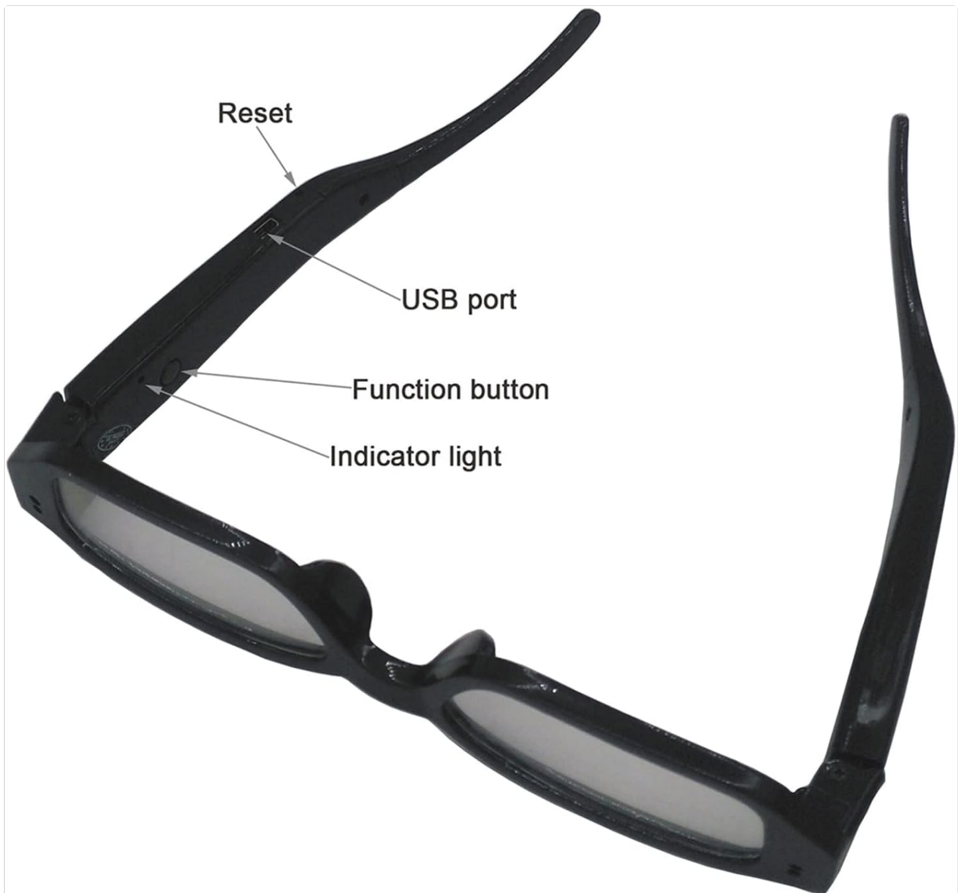
Figure 3.2: Side view of the glasses with key components labeled: USB port, function button, indicator light, and reset button.
