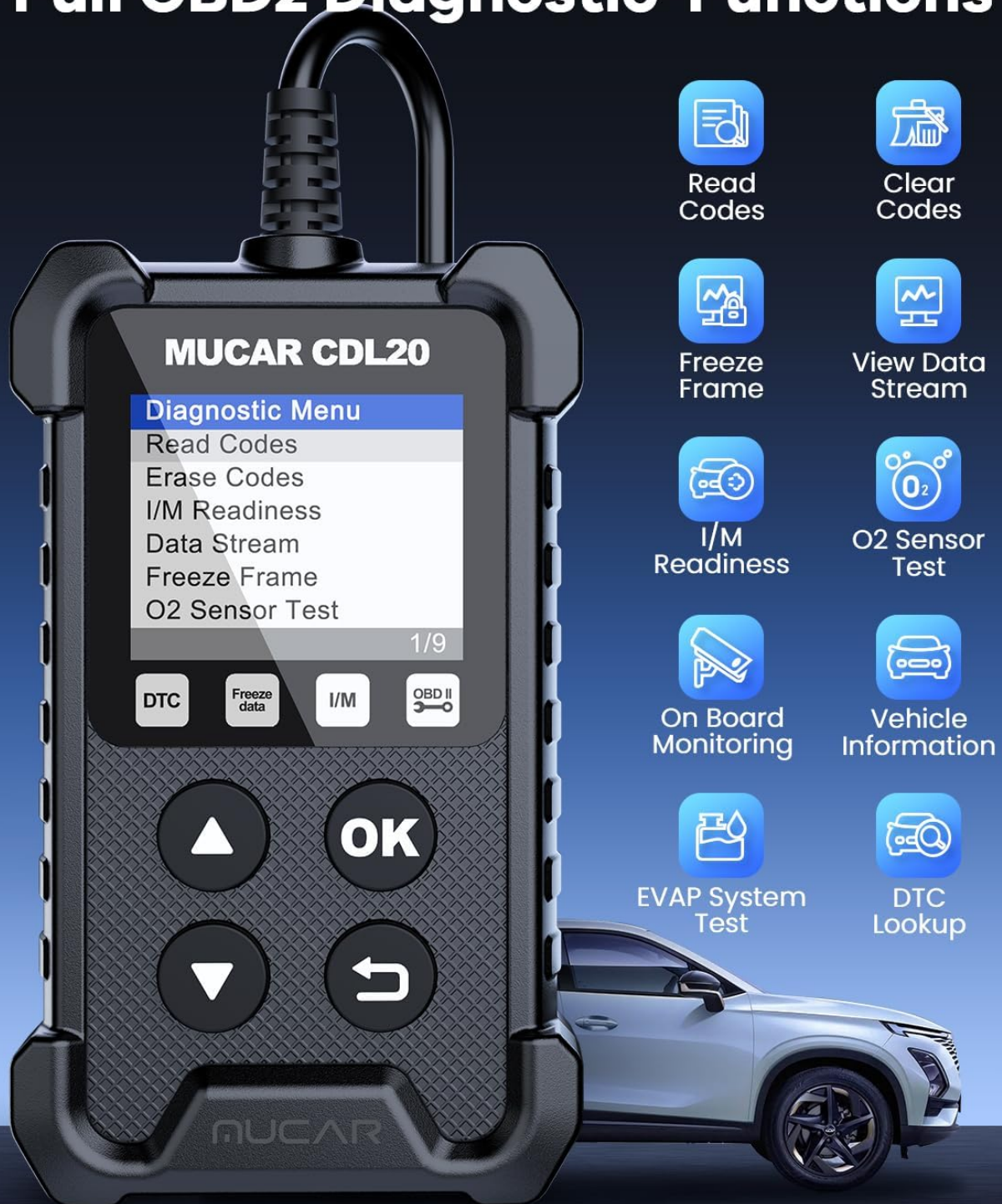
Image 2.2: MUCAR CDL20 OBD2 Scanner showing its main diagnostic menu with options like Read Codes, Erase Codes, I/M Readiness, and Data Stream.
