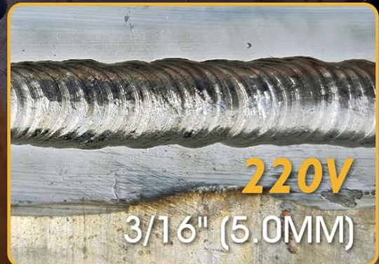
Figure 5.2: Aluminum welding thickness examples at different voltages.
