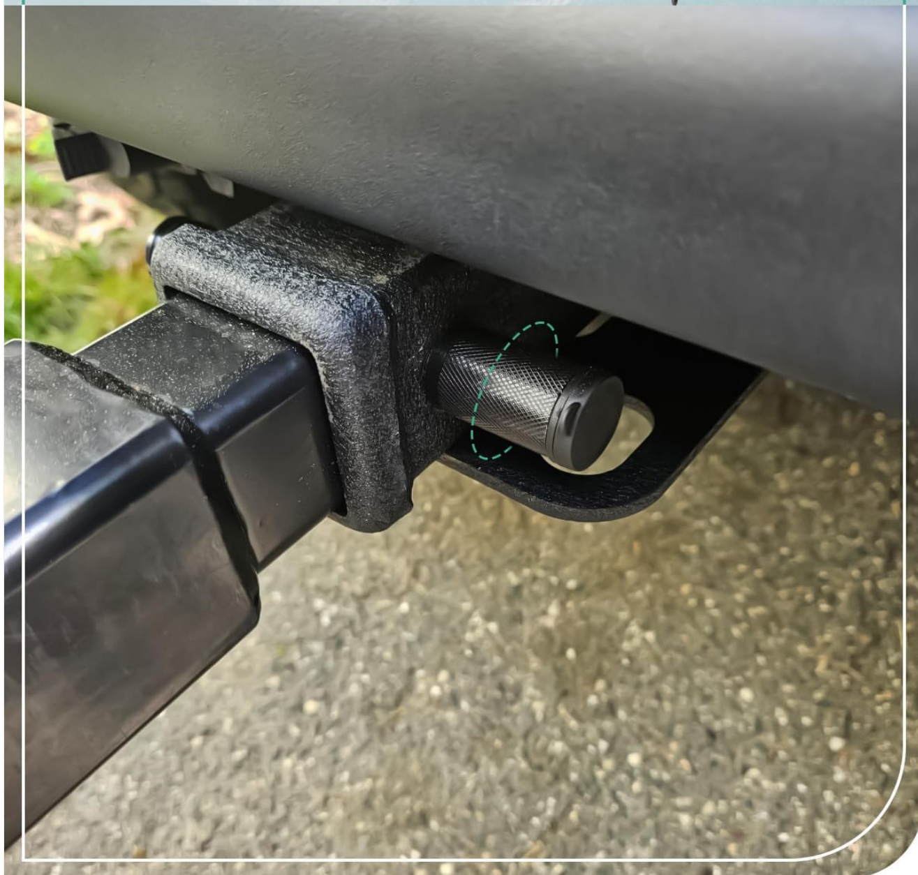
Figure 2: Secure the rack using the threaded hitch pin and anti-rattle insert.
