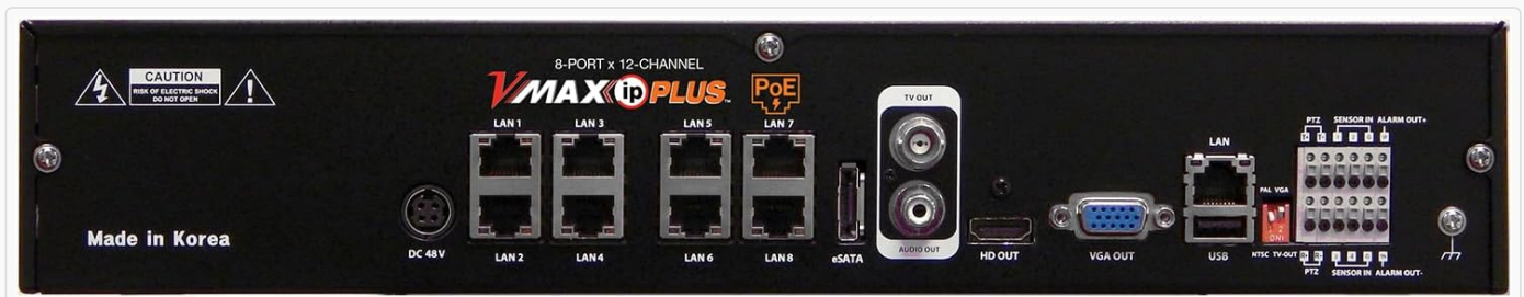
Figure 4.2: Rear view of the VMAX IP Plus NVR. This image illustrates the rear panel, highlighting the 8 PoE ports for direct camera connection, LAN ports, TV Out (BNC), Audio Out, HDMI Out, VGA Out, USB ports, and alarm input/output terminals.
