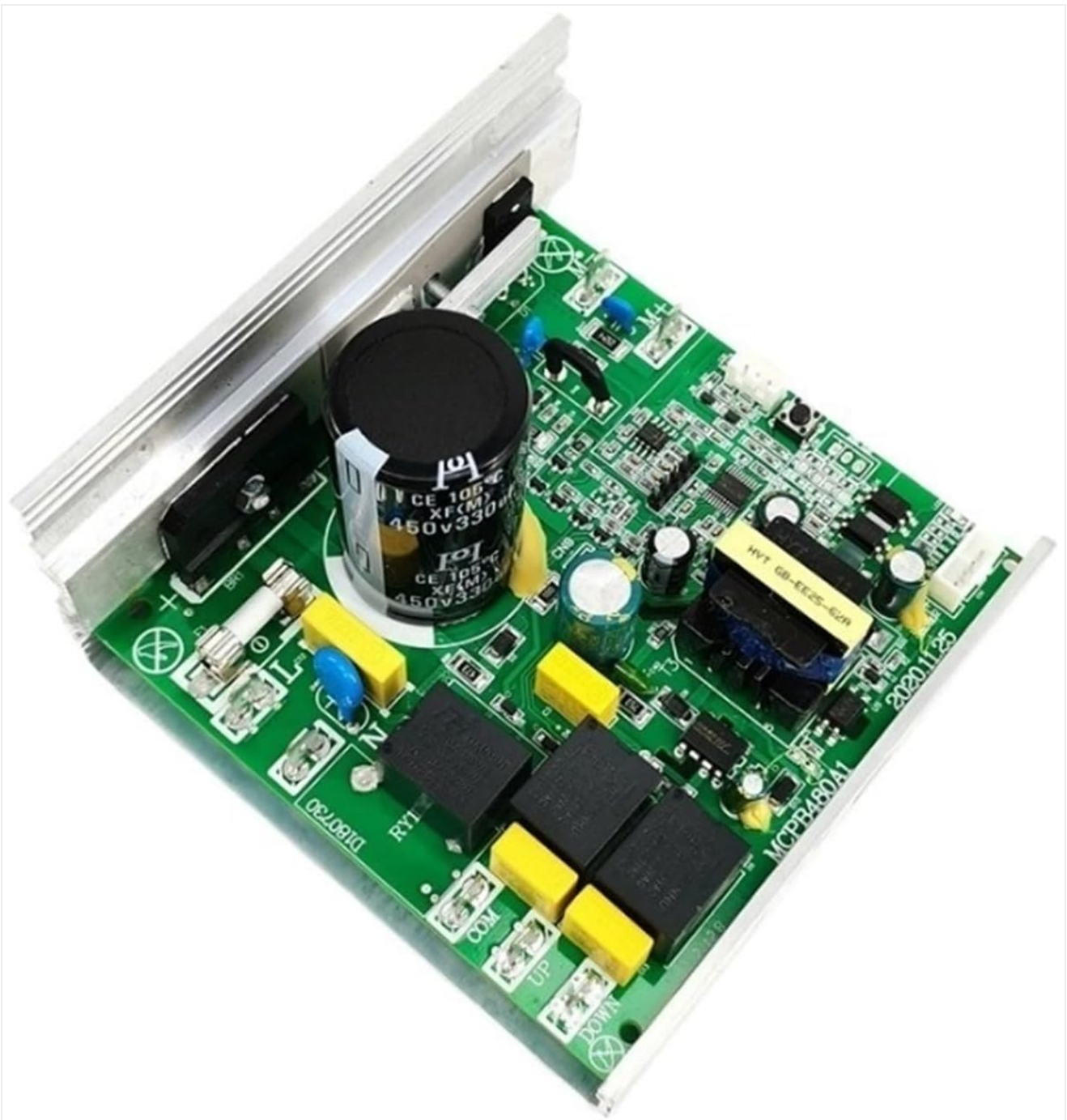
Figure 4: Side view of the MCPB480A1 controller, illustrating the heat sink for thermal management.
