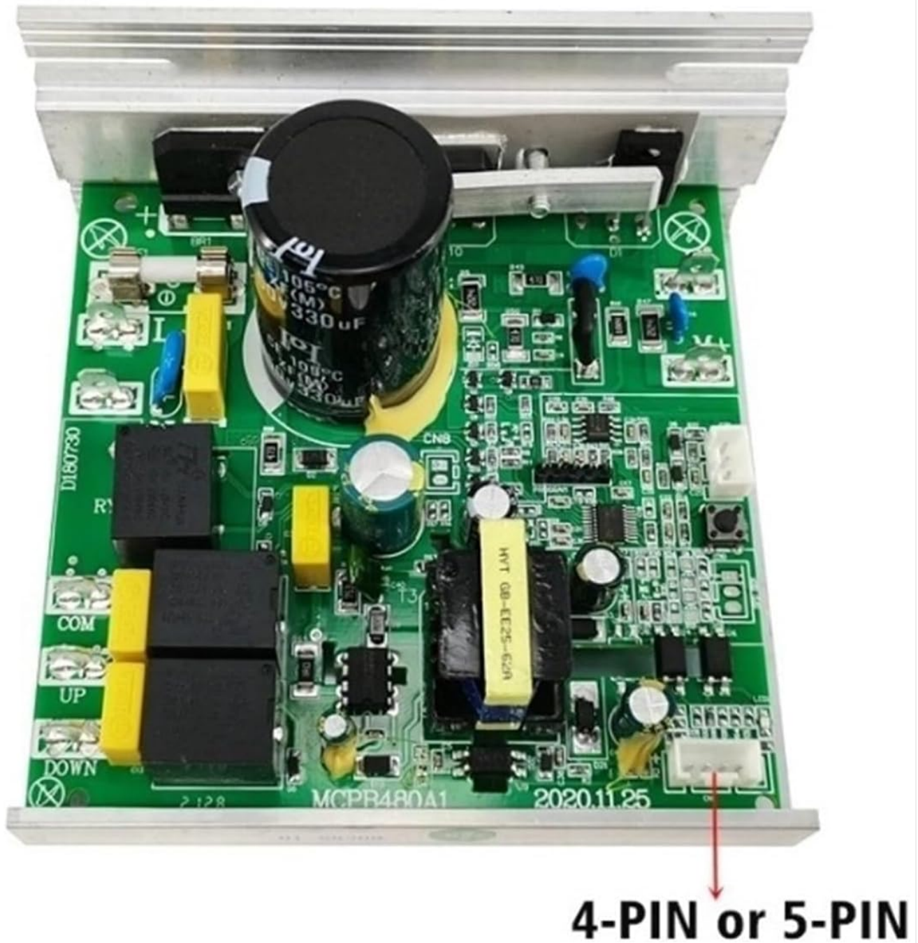
Figure 3: The MCPB480A1 board, indicating its compatibility with both 4-pin and 5-pin connections.
