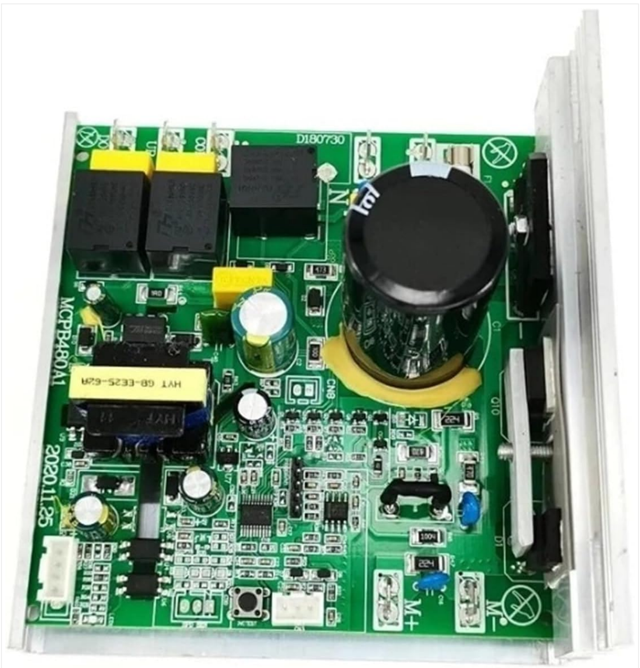
Figure 5: Top-down view of the MCPB480A1 controller board, showing component layout.
