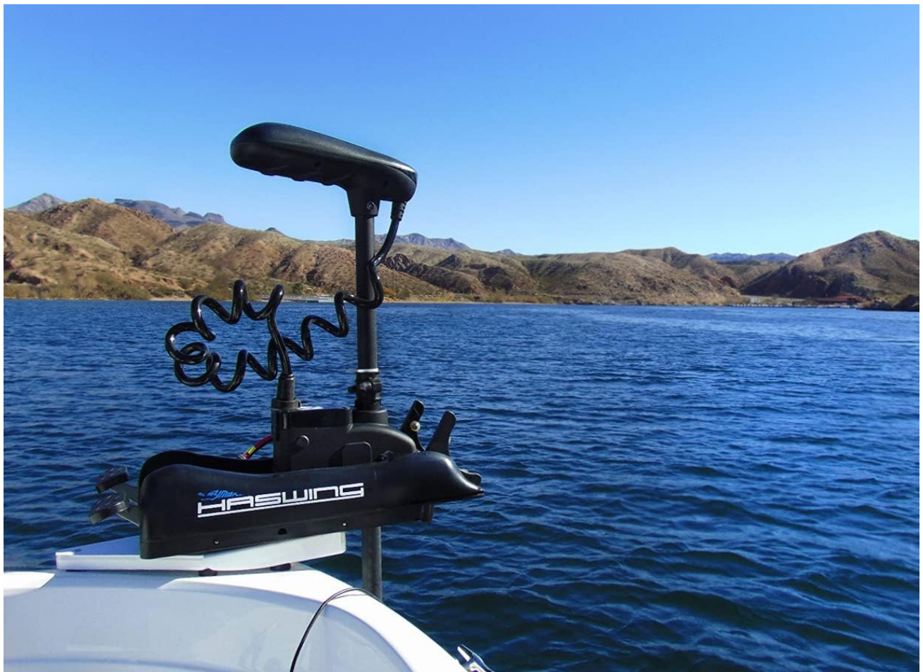
Figure 2.1: Detail of the bow mount mechanism.
