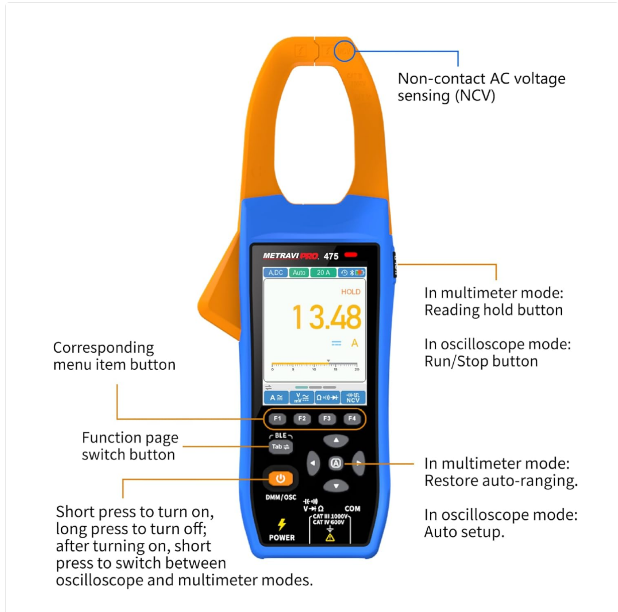
Image 6.1: Key operating controls of the Metravi PRO 475.
