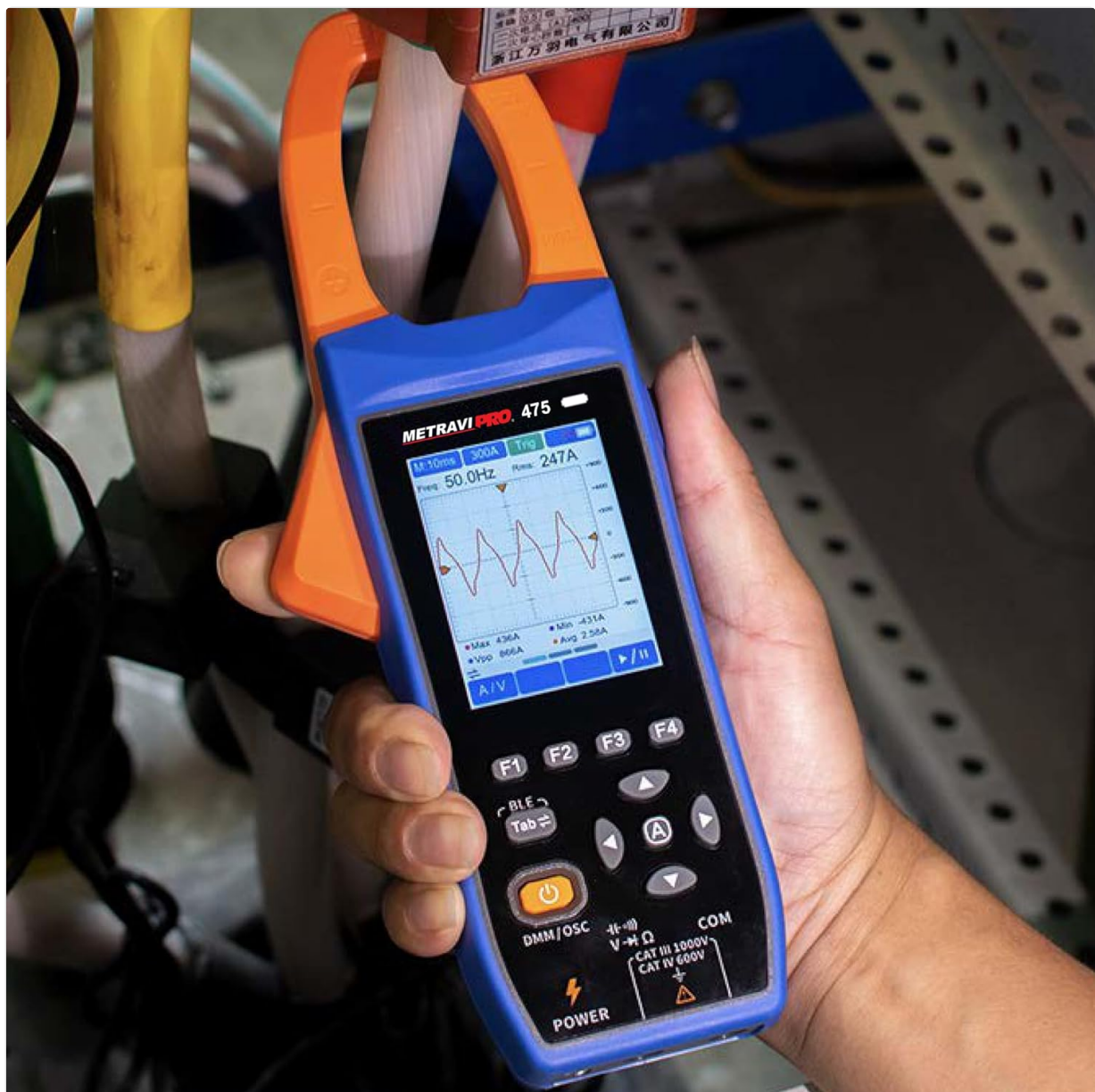
Image 6.3: Performing a current measurement with the clamp jaw.
