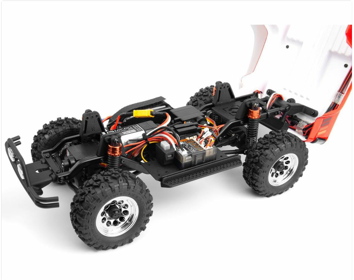
Image: Internal chassis and electronics layout of the Venture18 crawler.
