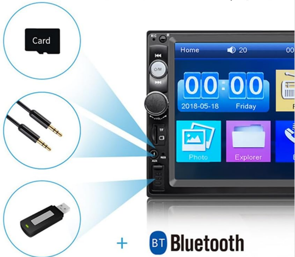
Figure 6.4: Visual representation of the four available playback modes: USB flash disk, AUX input, Bluetooth, and TF Card.
