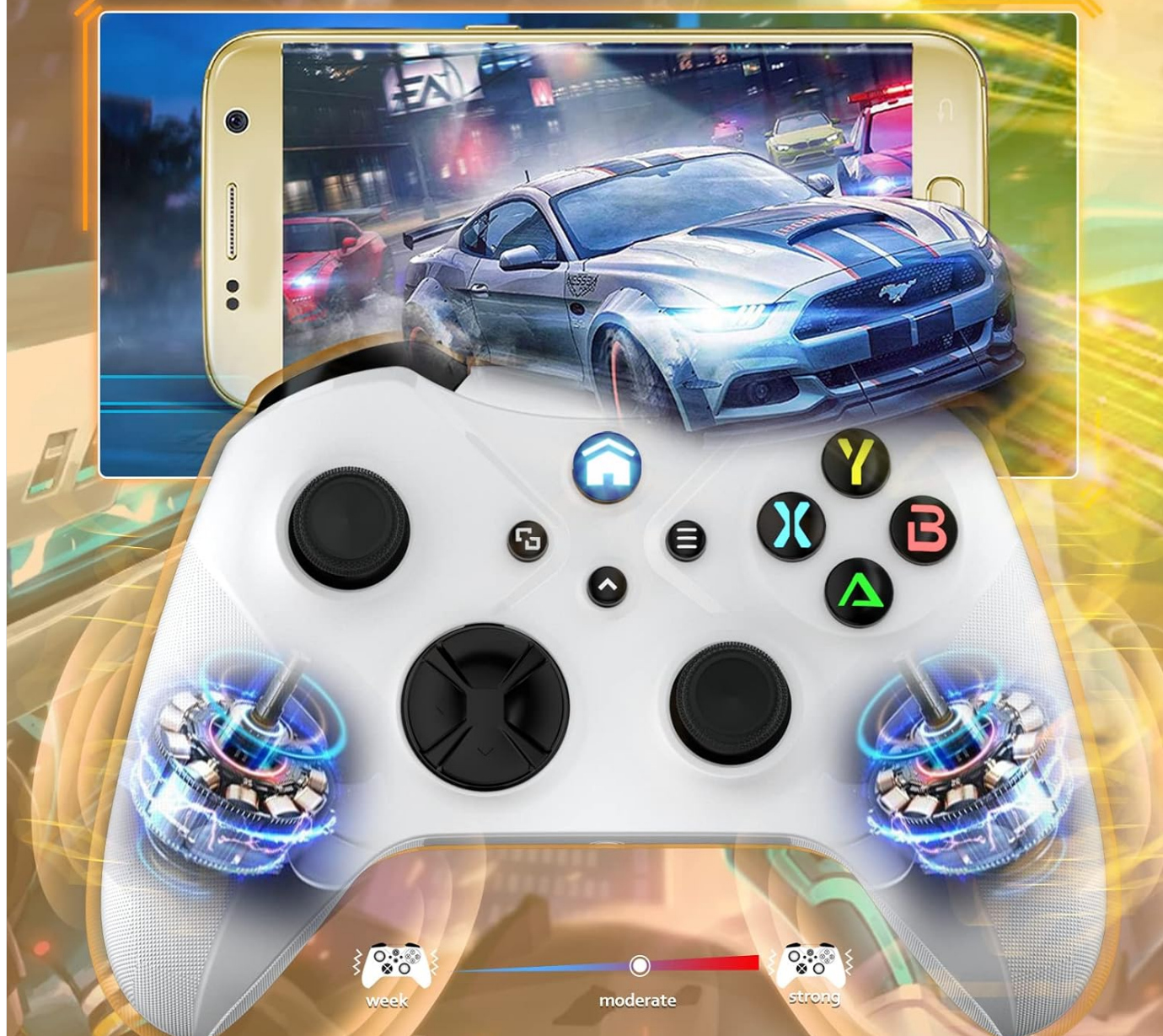
Figure 5: Illustration of the dual vibration motors providing haptic feedback.
