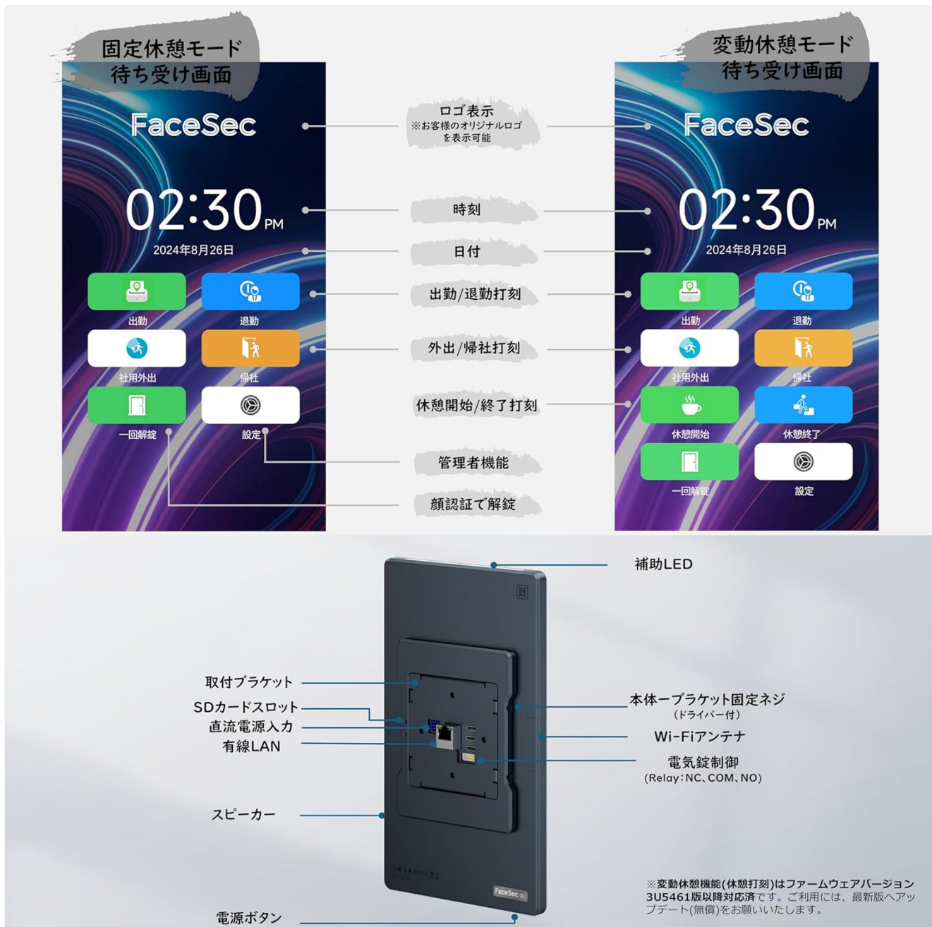
Image: This image displays the back panel of the FaceSec time recorder, highlighting the mounting bracket, SD card slot, DC power input, wired LAN port, Wi-Fi antenna, electric lock control (Relay-NC, COM, NO), and power button. It also shows a comparison of the fixed break mode and variable break mode interfaces on the device screen.
