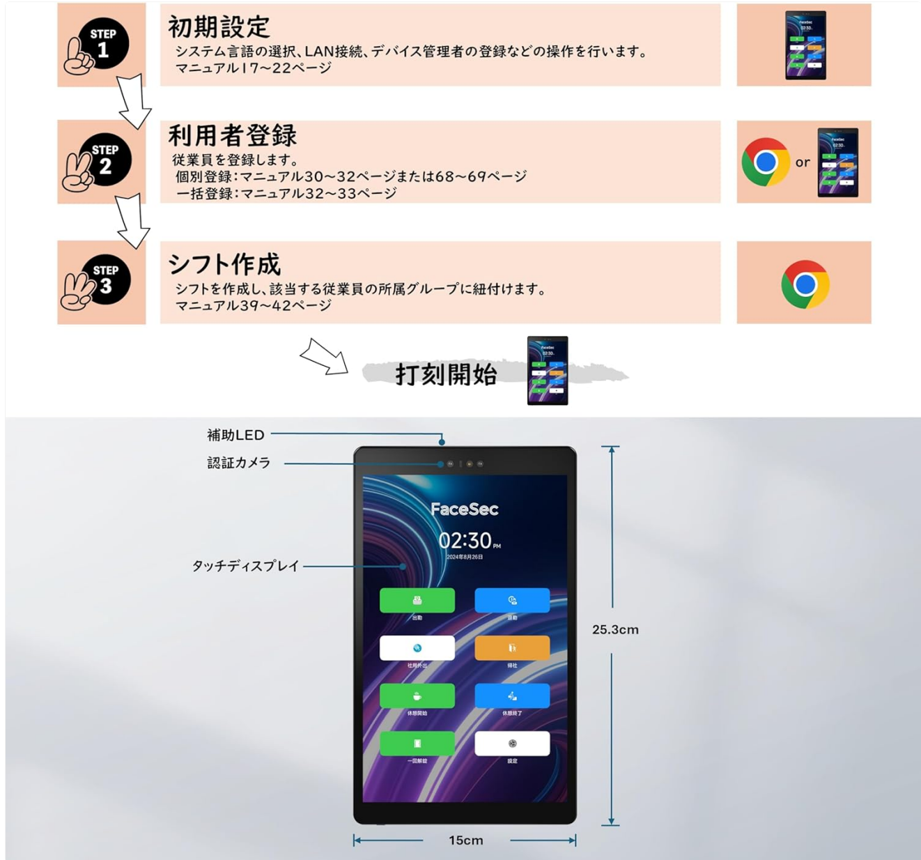
Image: Diagram illustrating the three main setup steps (Initial Setup, User Registration, Shift Creation) and the physical dimensions of the FaceSec time recorder. The device measures 25.3cm in height and 15cm in width, featuring an auxiliary LED, recognition camera, and touch display.
