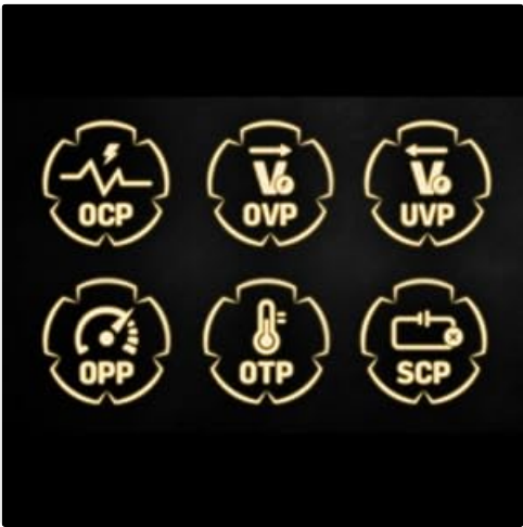
Image 6.1: Visual representation of the multiple protection circuitries integrated into the power supply for enhanced safety and component longevity.
