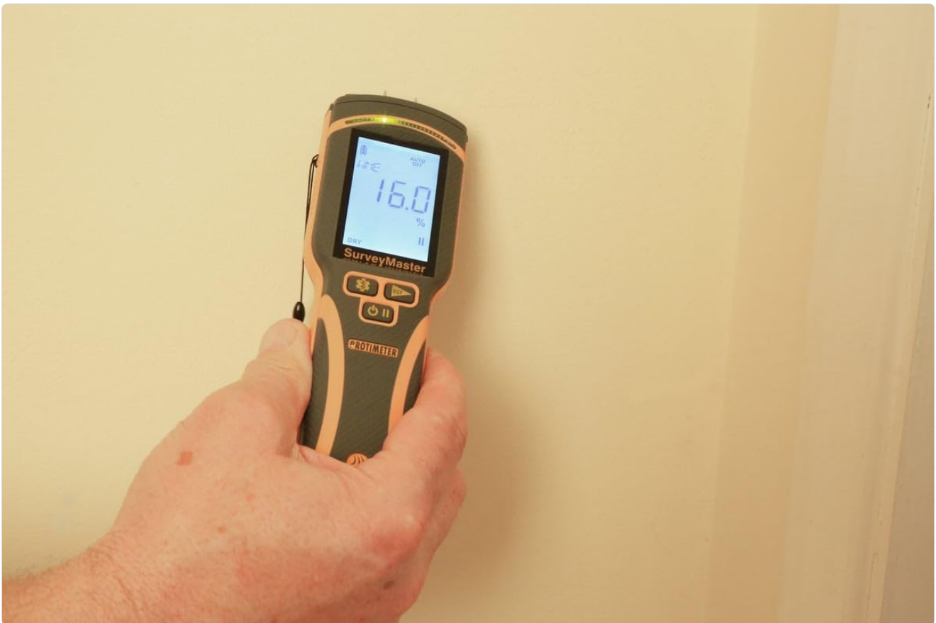
Figure 7: An inspector using the Protimeter SurveyMaster's integrated pins to measure moisture directly on a wall surface.
