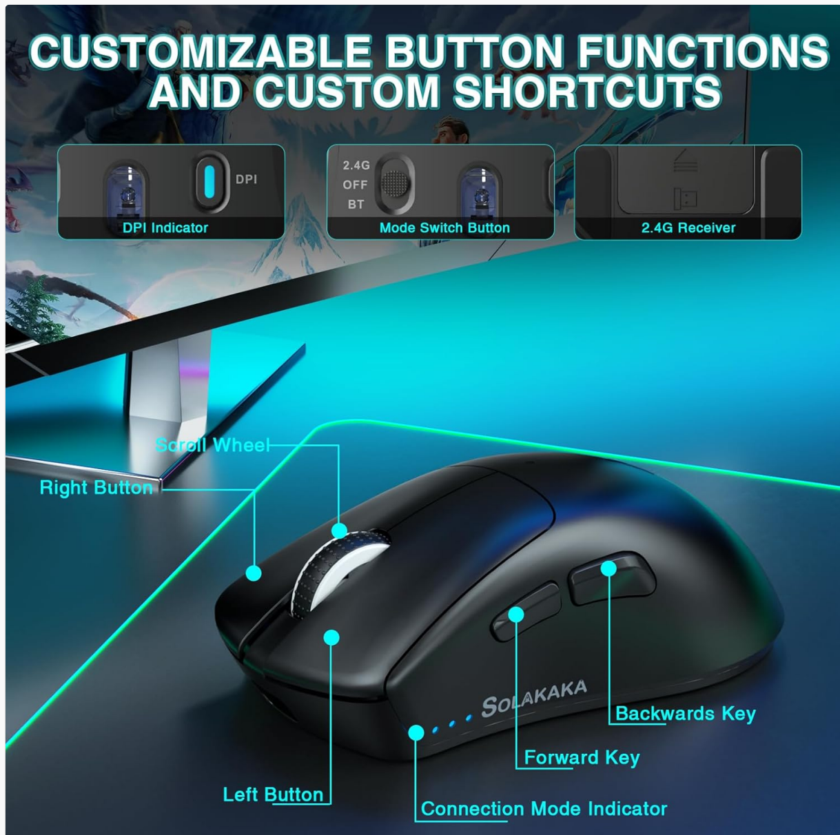
Figure 4: A detailed diagram pointing out the various buttons and indicators on the SM805 mouse, including the DPI
