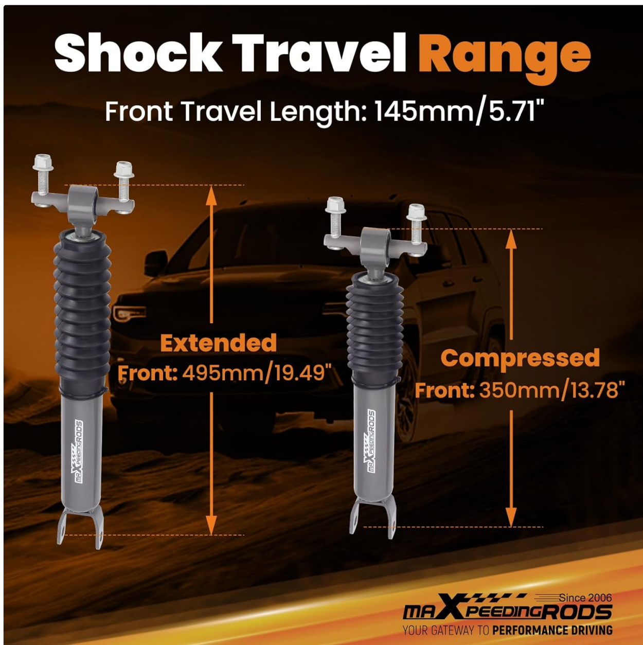
Image 4.1: Front Shock Absorber Travel Range.
