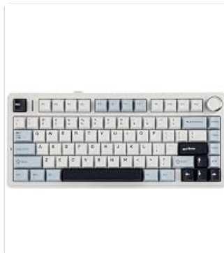
Figure 8: The HE68 features a hot-swappable PCB, allowing for easy replacement of magnetic switches.
