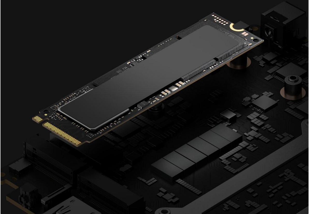
Image 6.1: An illustration of the expandable storage slot, indicating support for an additional M.2 NVMe PCIe 4.0 SSD.
