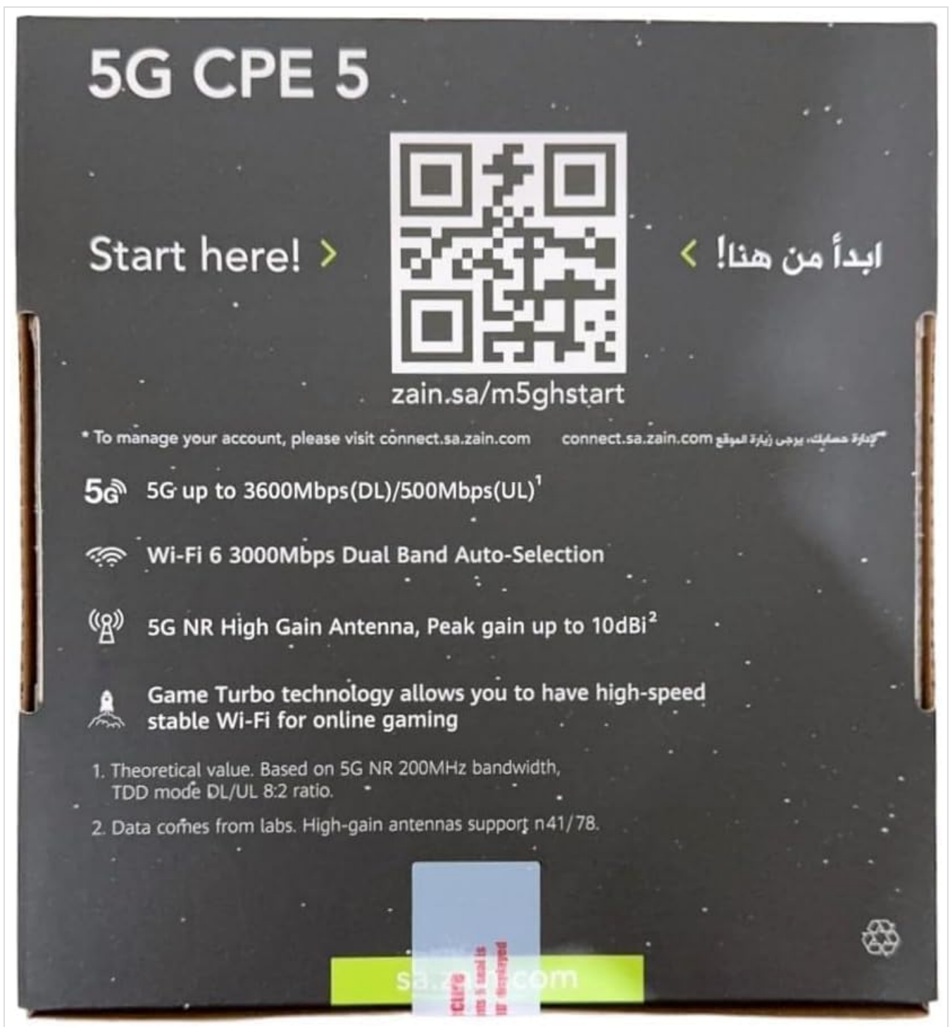
Figure 2.2.4: The bottom of the 5G CPE 5 Router H155-382 packaging, showing a QR code and text indicating the management portal address: zain.sa/m5ghstart . This section also details key performance metrics like 5G download/upload speeds and Wi-Fi 6 capabilities.
