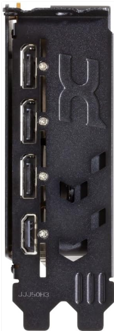
Figure 3: Side view of the graphics card, highlighting the display output ports (HDMI and DisplayPort).
