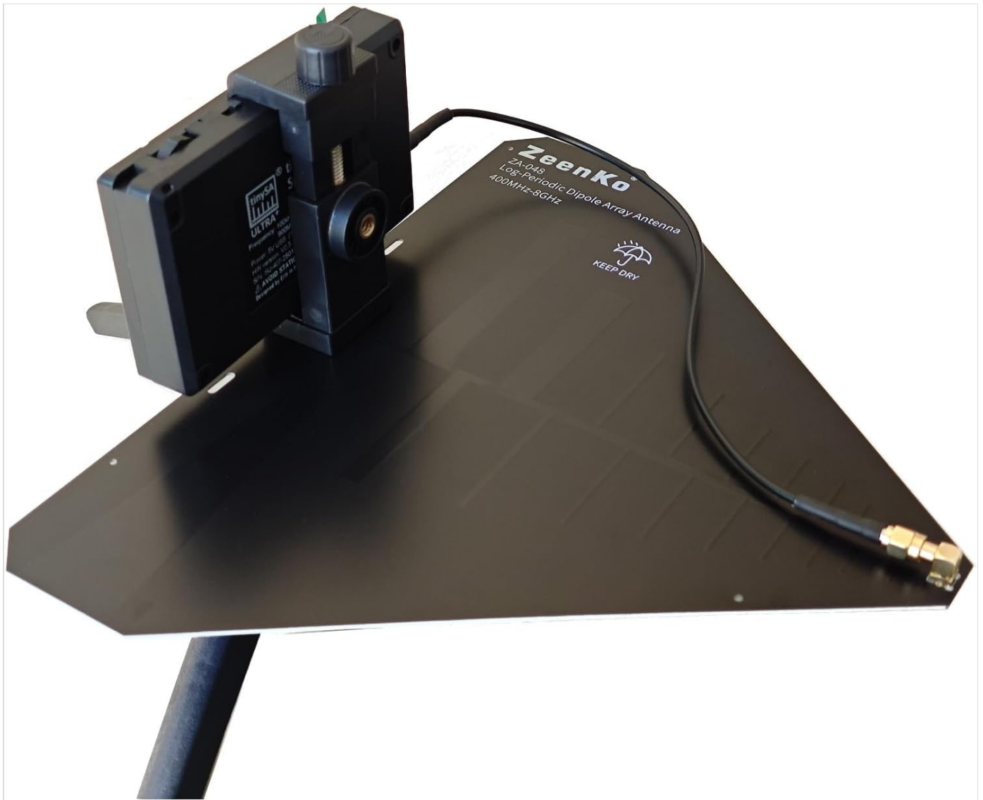
Figure 3.1: The ZA-048 antenna connected to a tinySA Ultra spectrum analyzer, mounted on a tripod for stable operation.
