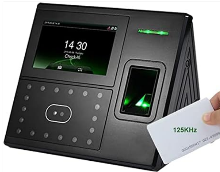
Figure 5: The NJBVRS UFace402 device demonstrating an optional card being scanned for user authentication or registration.
