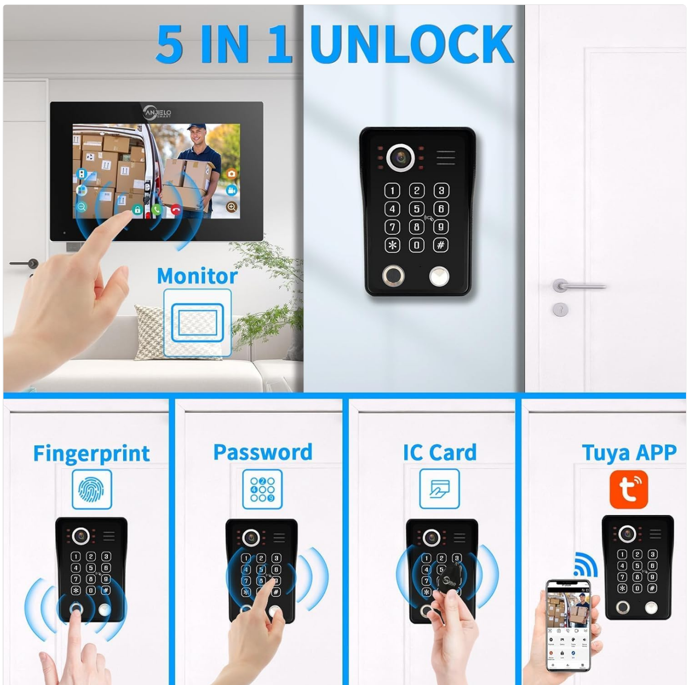
Figure 6.2: The five unlocking methods available.
