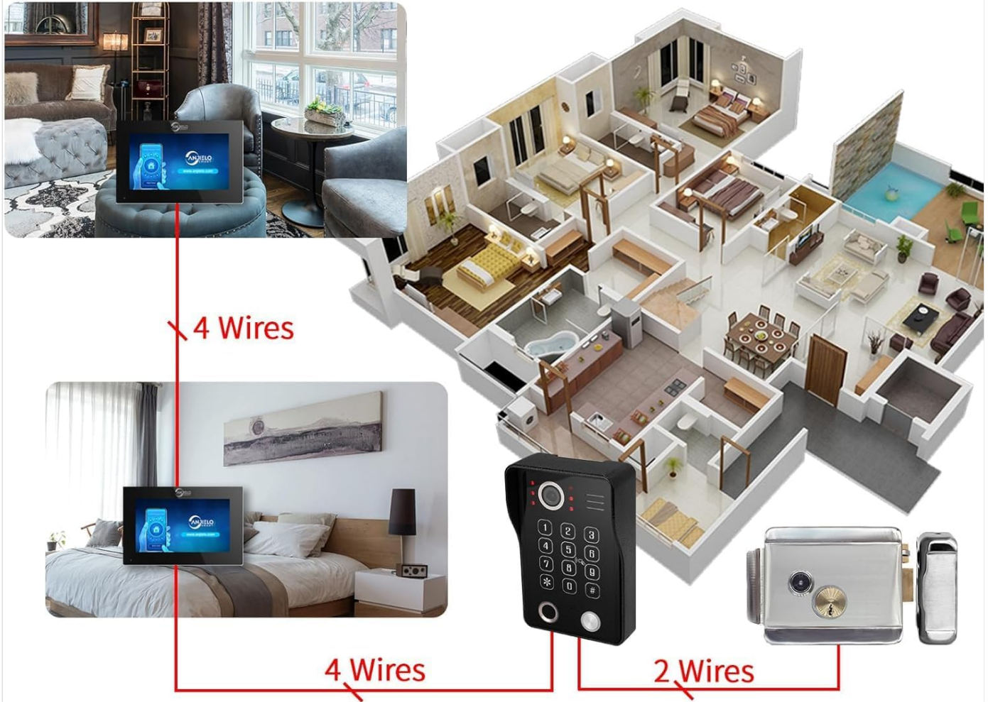
Figure 5.1: Wiring connections for the intercom system.
