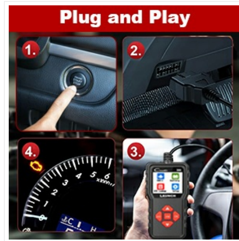
Figure 4.1: Illustration of the plug-and-play connection process. The image shows four steps: 1. Starting the car, 2. Plugging the OBDII connector into the vehicle's port, 3. The scanner displaying information, and 4. The check engine light on the dashboard.
