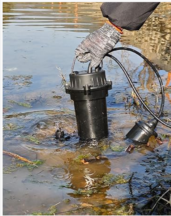
Figure 2.1: Always lift the pump by its handle. Never pull the power cord.
