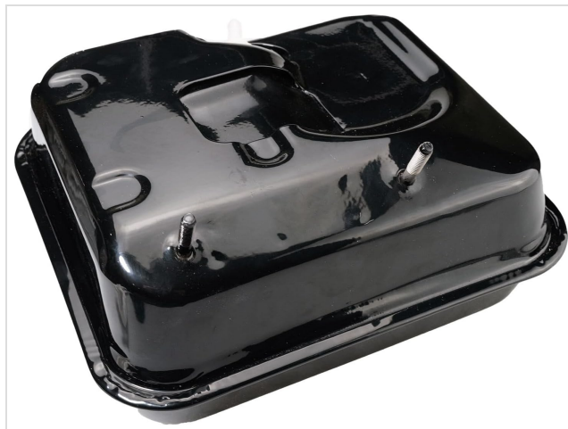
Image 5.1: Top view of the fuel tank, highlighting the mounting studs and fuel cap opening.
