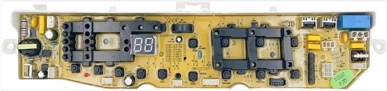
Figure 3.1: Top view of the Lfidontkl Samsung Washing Machine Control Board, showing the main circuit layout and connectors.
