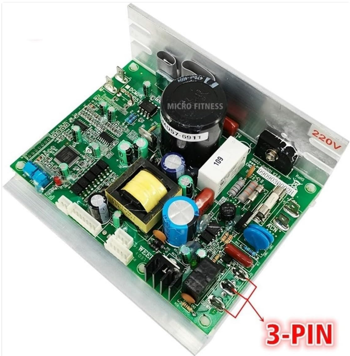
Figure 1: General view of the SQJZWOD DCMD57 series treadmill control board, highlighting the 3-pin power connection.
