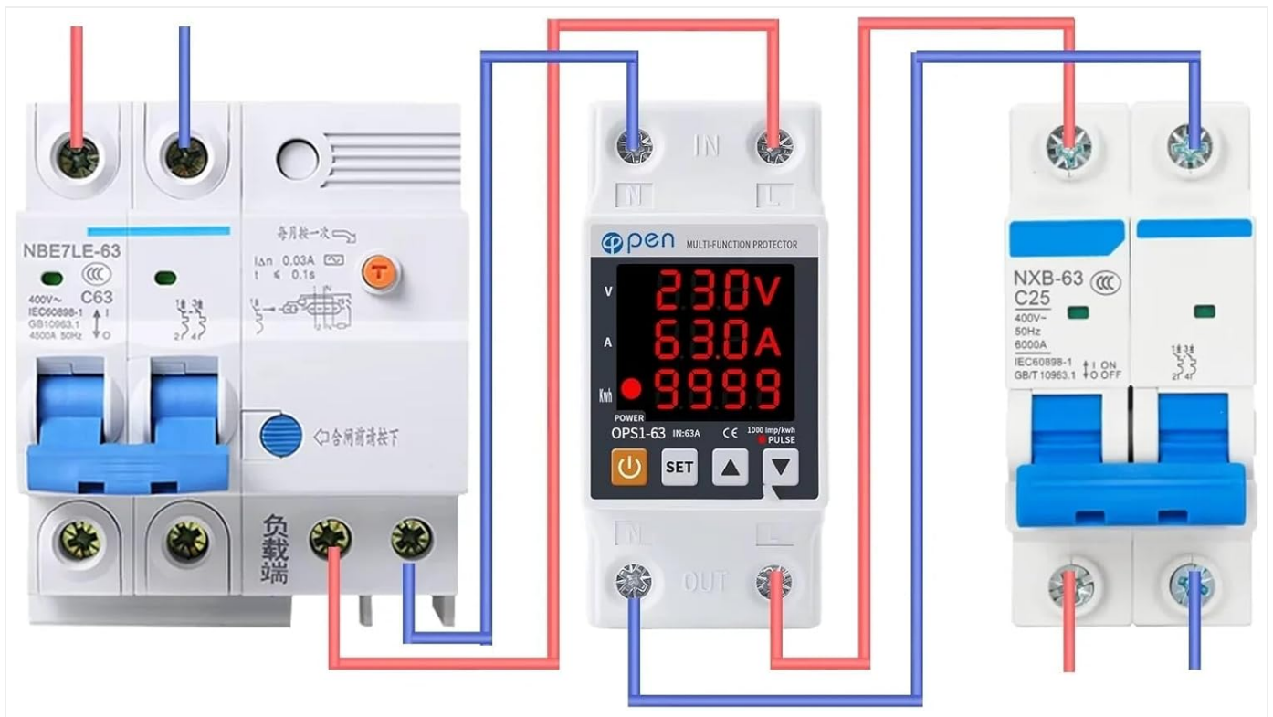
Figure 5.2: Wiring diagram. The diagram illustrates connecting the device between an incoming power source (left circuit breaker) and the protected load (right circuit breaker). Input terminals are marked 'IN' and output terminals 'OUT'. After wiring, double-check all connections for tightness and correctness before restoring power.
