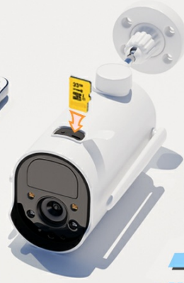
Image 4.4: The camera supports both cloud and Micro SD card storage for video recordings.
