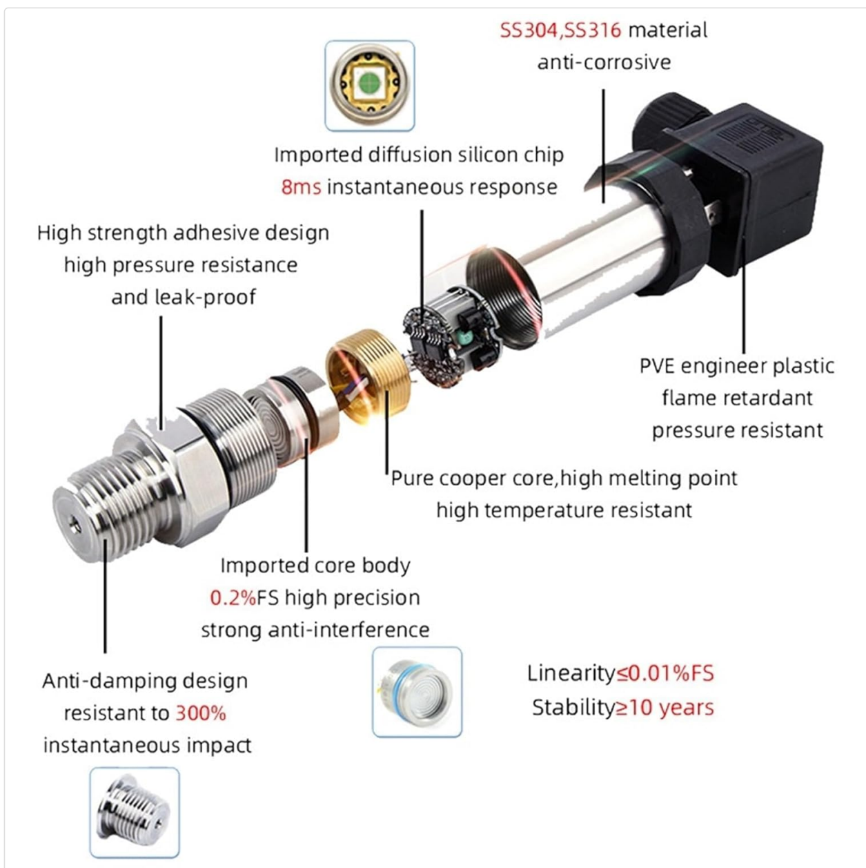
Figure 2: Exploded view of the QDW90A Pressure Transmitter. This diagram illustrates the internal components, including the SS304/SS316 anti-corrosive material, imported diffusion silicon chip with 8ms response, high strength adhesive design, PVE engineer plastic flame retardant shell, pure copper core, and imported core body with 0.2%FS high precision and strong anti-interference capabilities. It also highlights the anti-damping design and linearity/stability specifications.
