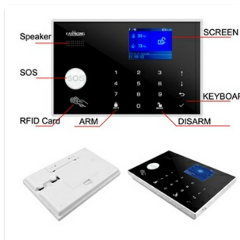
Figure 2.2: Detailed view of the main alarm panel features.
