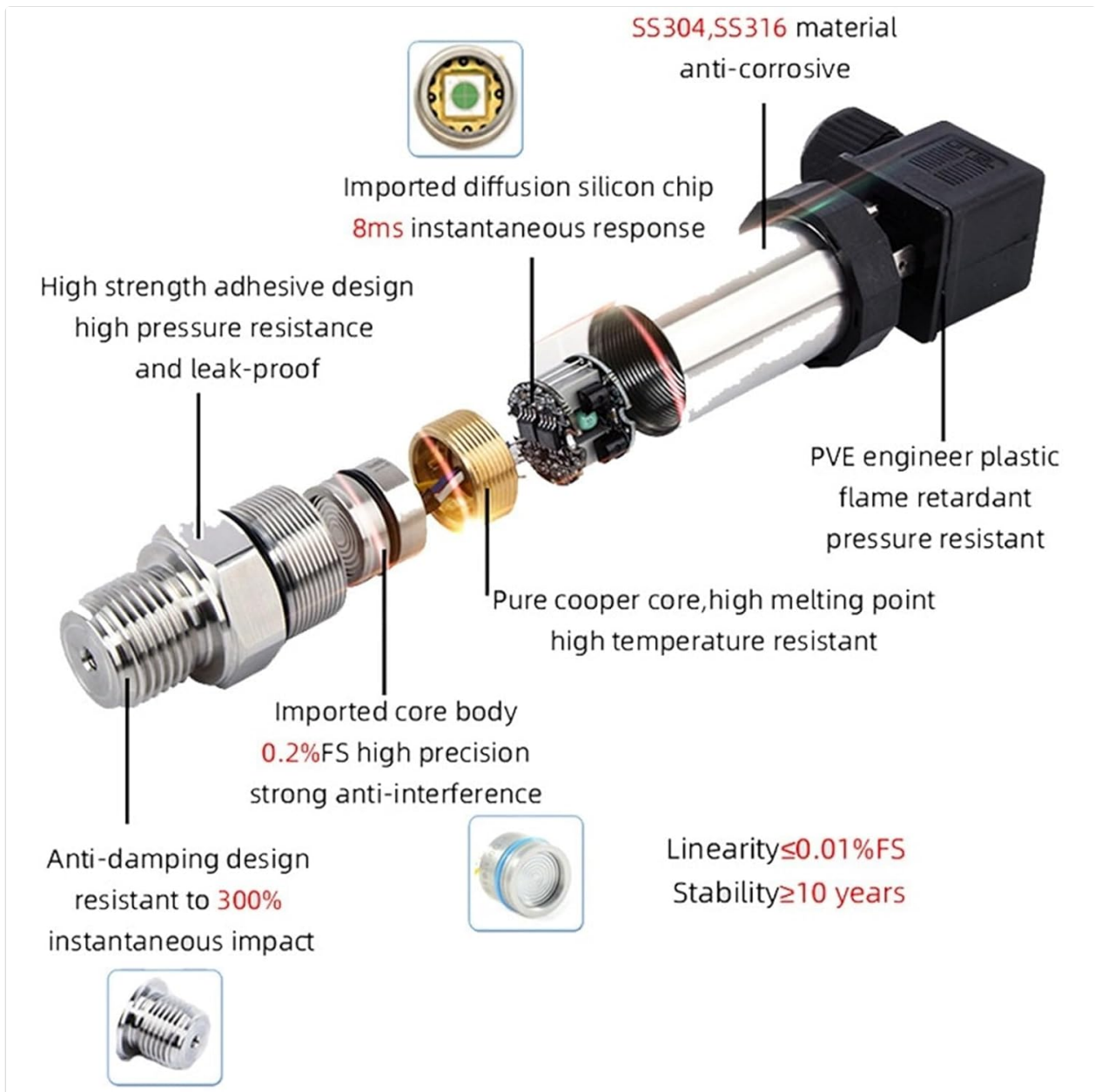
Figure 2: Exploded view illustrating the internal components and materials of the QDW90A Pressure Transmitter.
