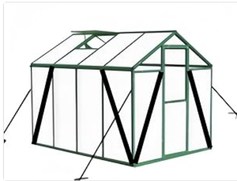
Image: Diagram showing the wind protection upgrades and anchoring points.
