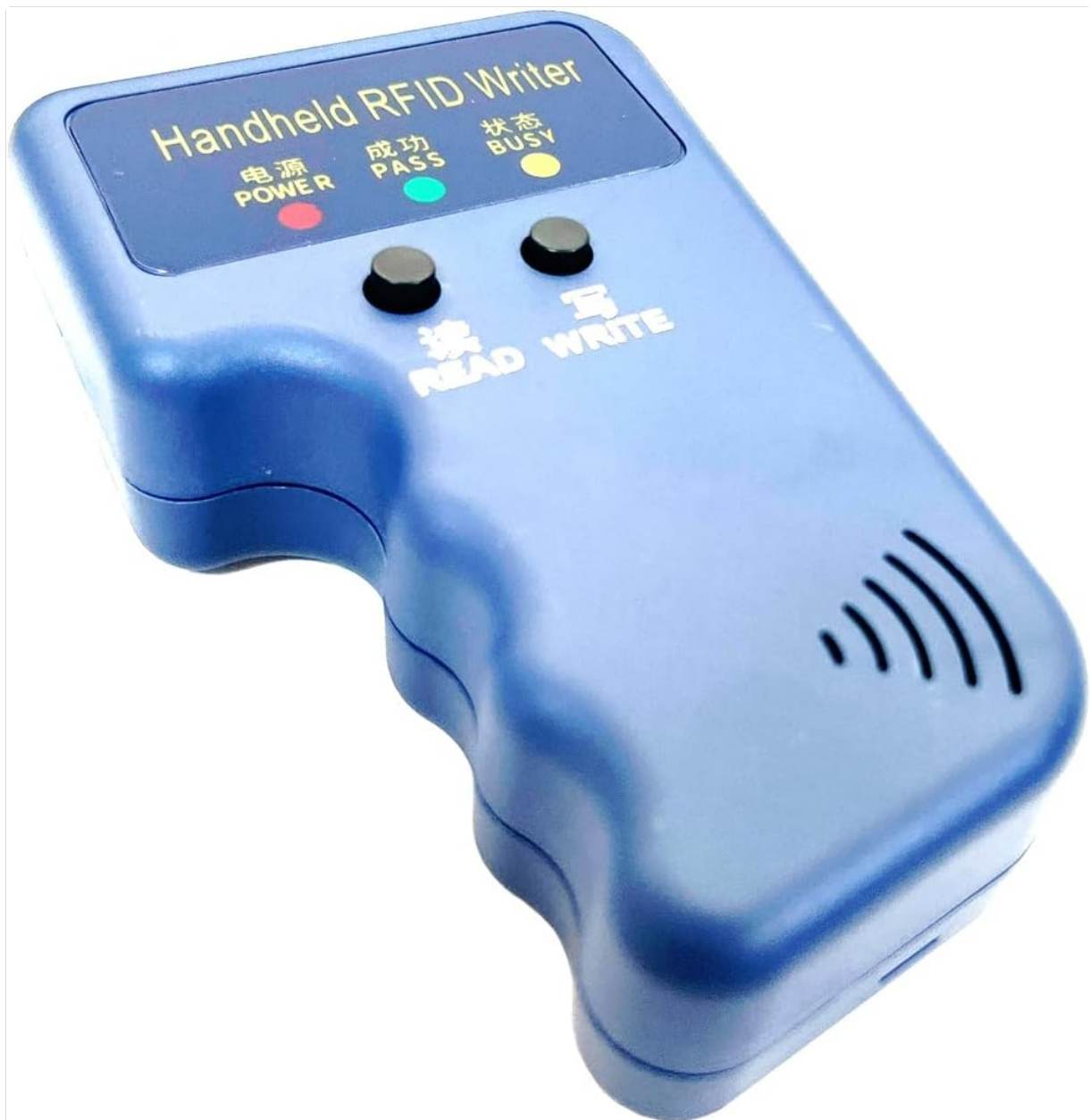
Image: The front panel of the RFID copier, clearly showing the "READ" and "WRITE" buttons, along with the "POWER", "PASS", and "BUSY" indicator LEDs.
