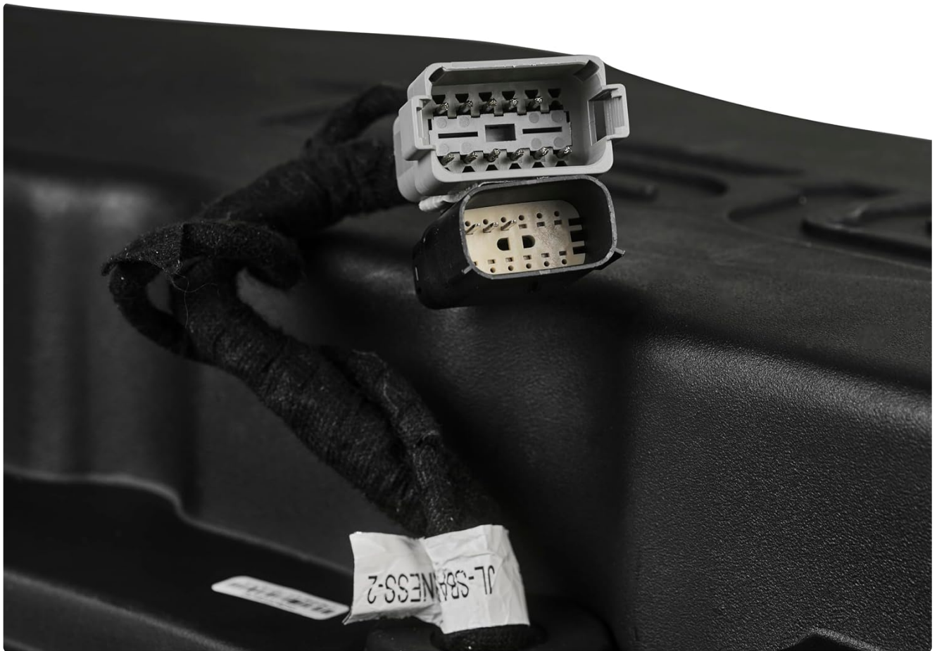
Figure 3: Ensure the wire harness is securely connected to the sound bar.
