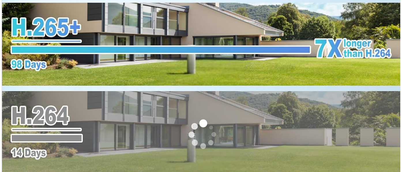
Figure 3.5: Comparison illustrating that H.265+ compression saves approximately 50% more storage space than H.264, allowing for significantly longer recording durations (e.g., 98 days vs. 14 days).
