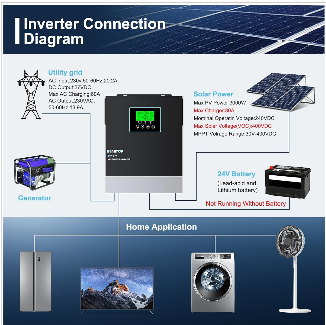
Image 4.1: Detailed connection diagram illustrating how to connect the inverter to the utility grid, solar panels, 24V battery, generator, and various home appliances. Note: The system requires a 24V battery to function.
