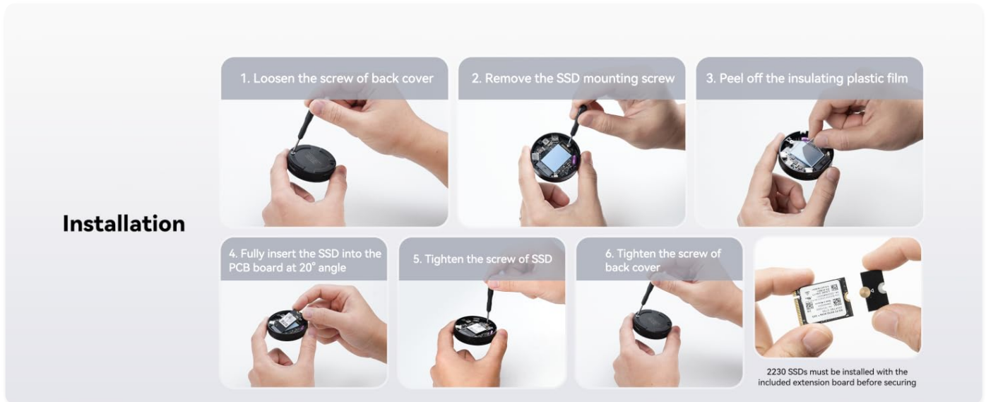
Image: Illustrated steps for installing an M.2 NVMe SSD into the DOCKCASE enclosure.
