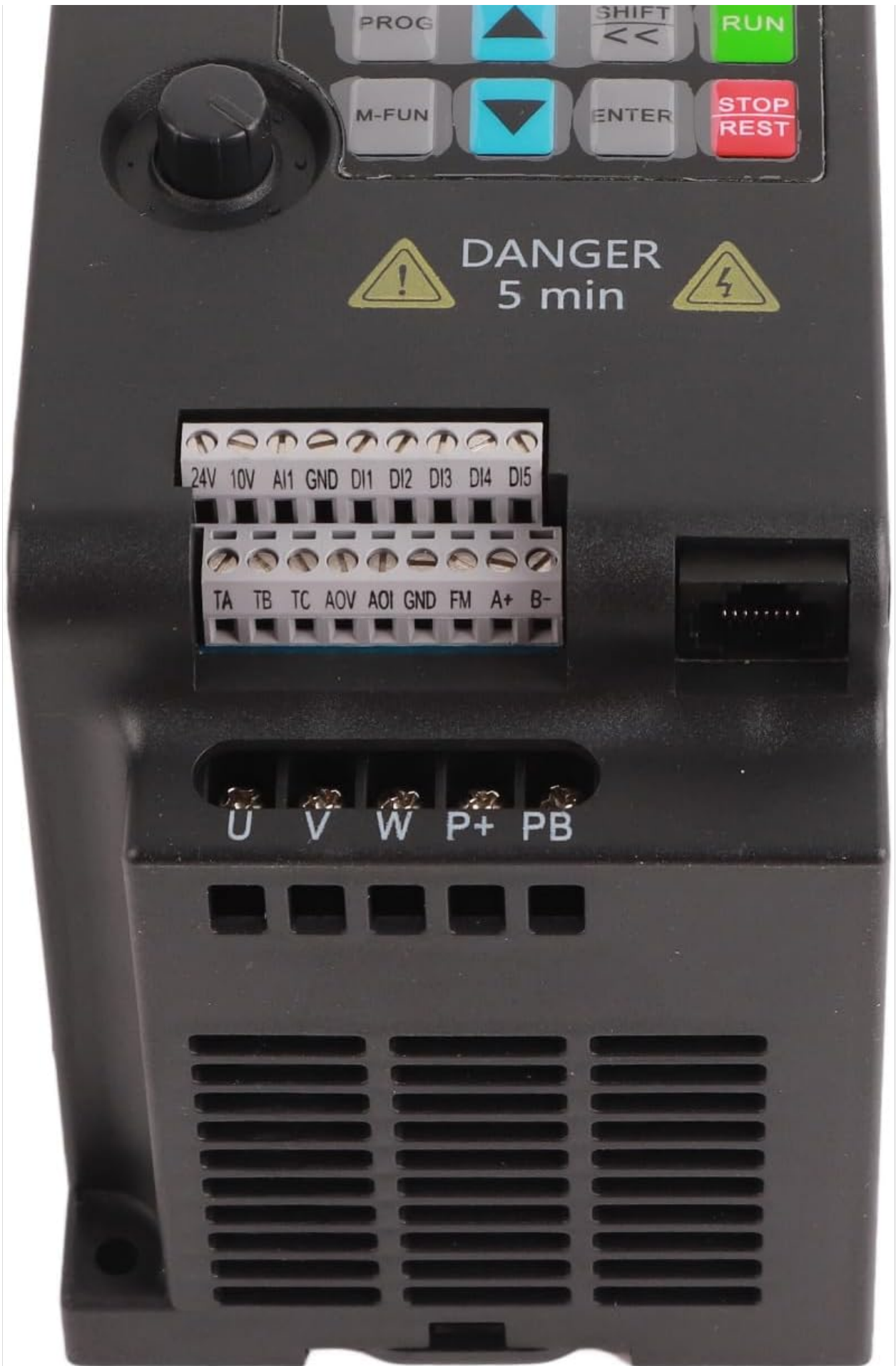
Figure 5.2: Top-down view of the VFD's terminal blocks, showing input (R, S, T), output (U, V, W), braking (P+, PB), and control terminals (24V, 10V, AI1, GND, DI1-DI5, TA, TB, TC, AO1, FM, A+, B-).
