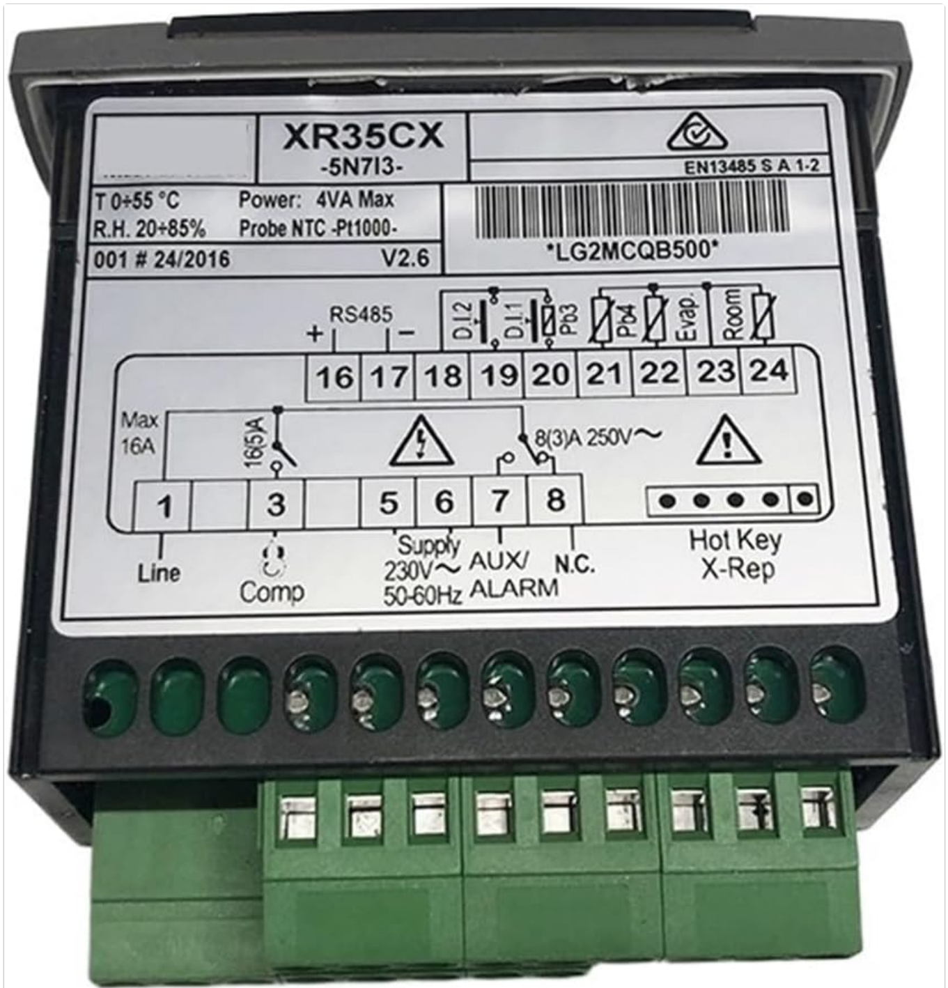
Figure 2: Rear view of the Aoleaby XR35CX-5N7I3 Temperature Controller, displaying the wiring diagram and terminal blocks. Key labels include "Line", "Comp", "Supply", "AUX/ALARM", "N.C.", "Hot Key X-Rep", and probe connections for NTC-Pt1000.
