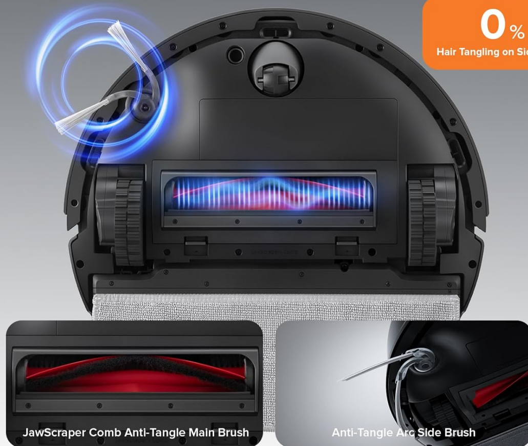
Figure 4.3: Close-up view of the dual anti-tangle system, showing the main brush and side brush designed to prevent hair tangling.
