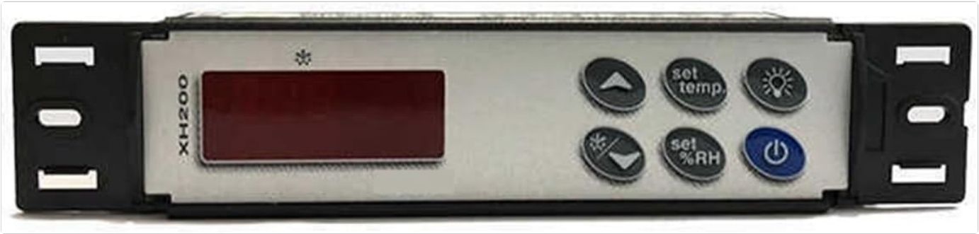
Figure 3.2: Close-up of the controller's front panel, featuring a red digital display on the left and six control buttons on the right. Buttons include 'Up', 'Set Temp', 'Light', 'Down', 'Set %RH', and 'Power'.
