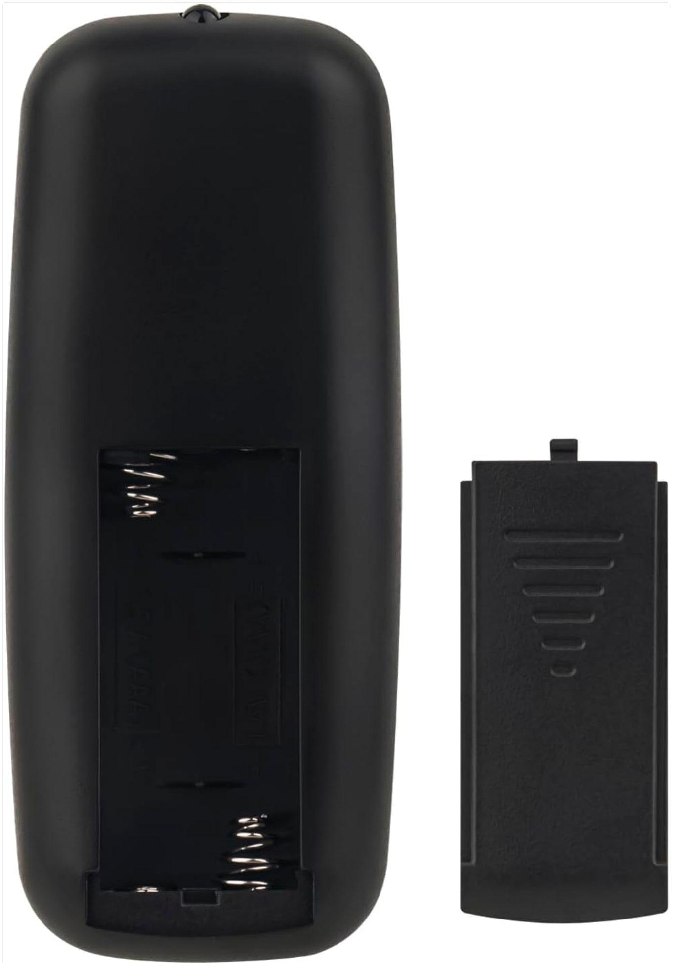
Figure 2.1: Rear view of the remote control with the battery compartment open, showing the two AAA battery slots.
