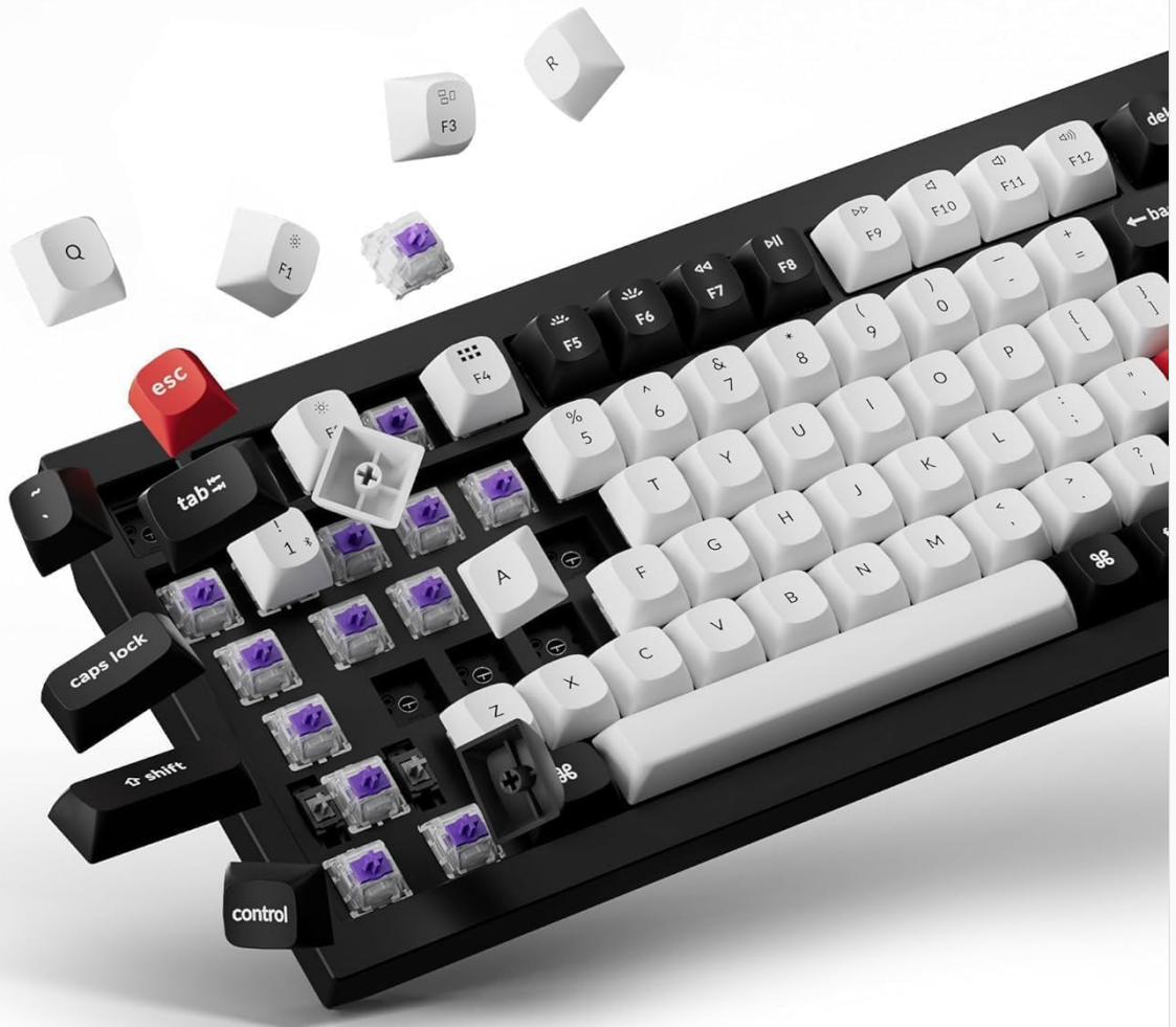
Image: A dynamic shot showing keycaps and magnetic switches being removed from the Keychron Q6 HE keyboard, highlighting its hot-swappable feature.
