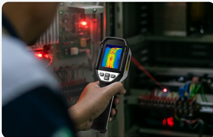
Image: A user aiming the thermal camera, demonstrating the laser-assisted autofocus feature.
